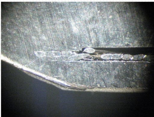
Wire braid welding
