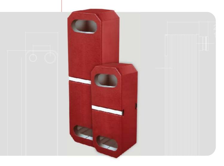
This insulation for heating applications consists of 2 half-shells and is made of FCKW-free polyurethane-foam with PS-folia. Due to the half-shell system, the assembly on the already installed heat exchanger is possible.
